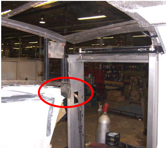
Figure 6: Connection of bus body to driver's cabin curb side
